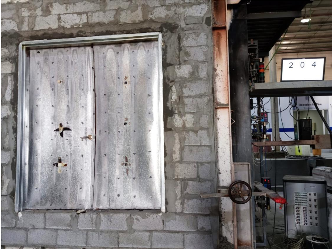
Figure 7: The end of the fire endurance test after 120 minutes.
