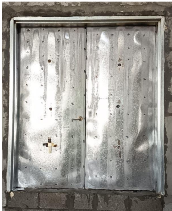
Figure 13: The unexposed face after the test.
