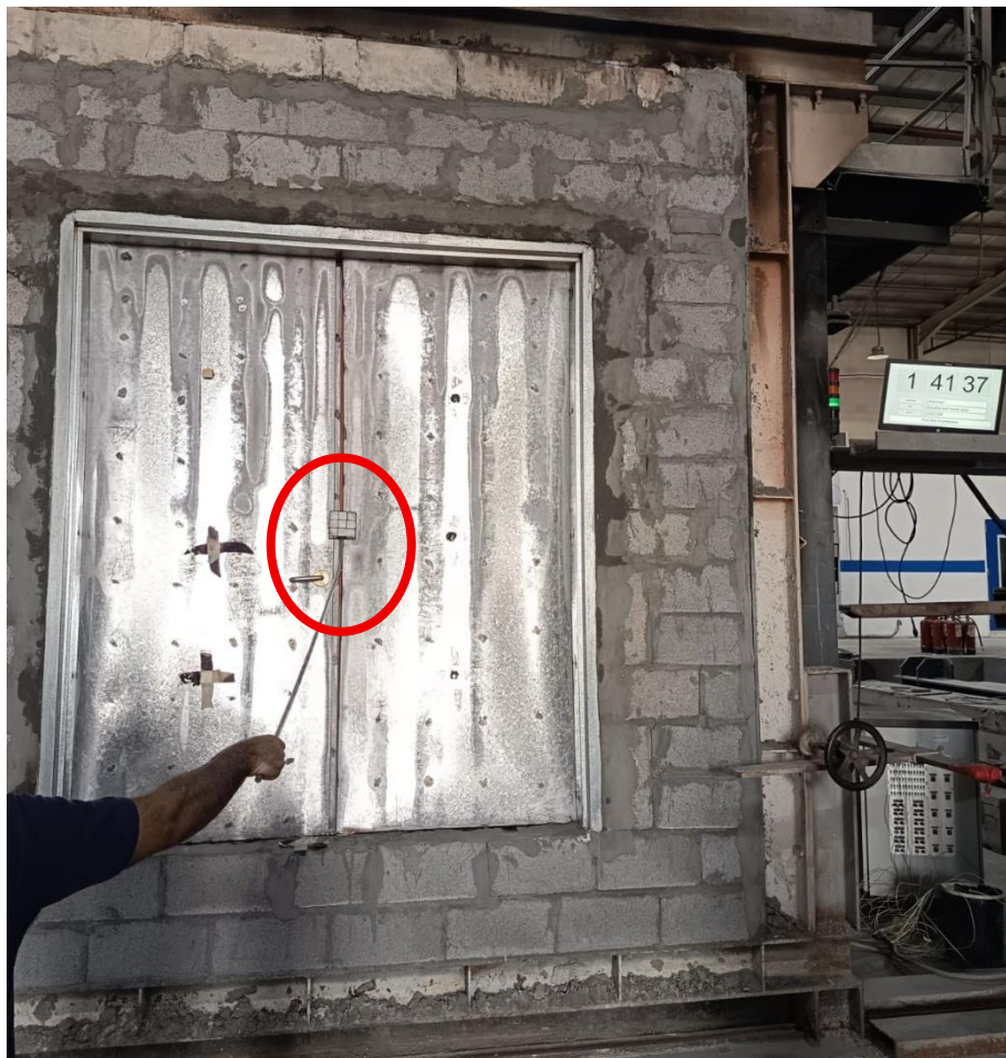
Figure 6: Application of cotton bad after 100 minutes of fire exposure (no ignition).
