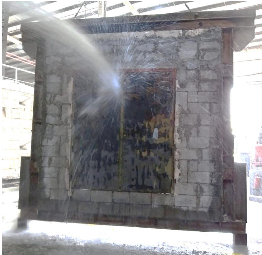
Figure 9: Hose stream test after 120 minutes of fire endurance
