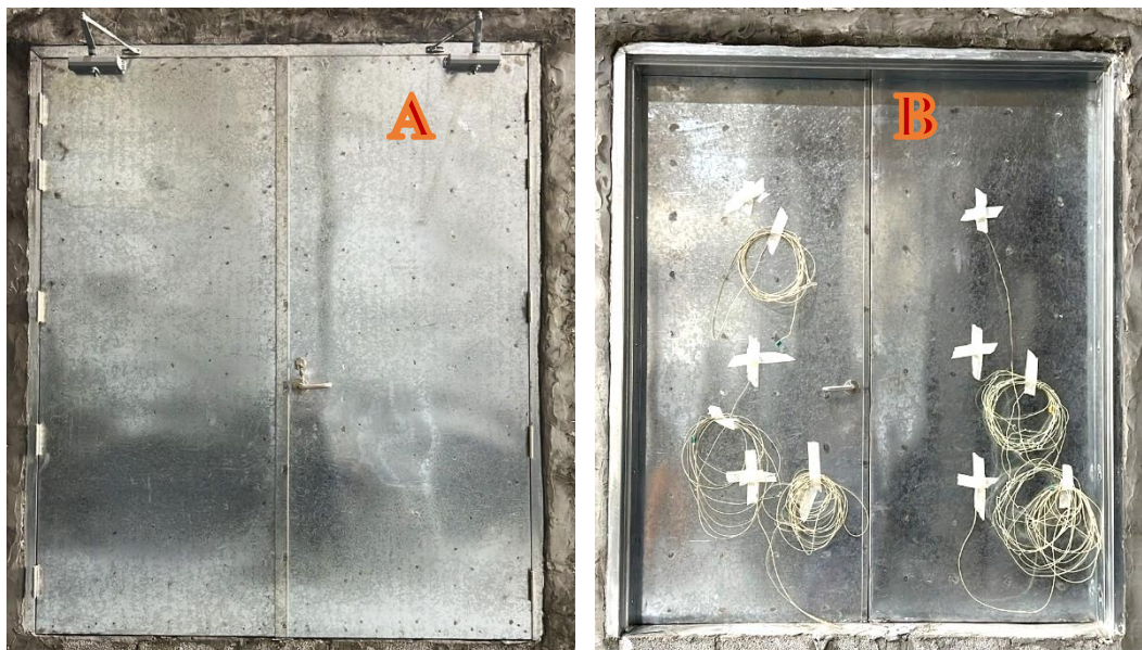
Figure 1: Photos of the door assembly, (A) Exposed face, (B) Unexposed face
